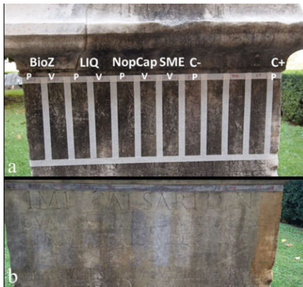
Fig. 11.5 Biofilm removal on marble artifact at Diocleziano Termae, Rome. (a) shows the scheme of the trial, with the product applied in cellulose pulp (P) and in Vanzan gel (V). From left to right: BioZ in cellulose pulp and Vanzan, LIQ in cellulose pulp and Vanzan, NopalCap in cellulose pulp and Vanzan, SME1.11 in Vanzan, C- (water in cellulose pulp) and C+ (benzalkonium chloride 1% in cellulose pulp). (b) the result soon after the pack removal
