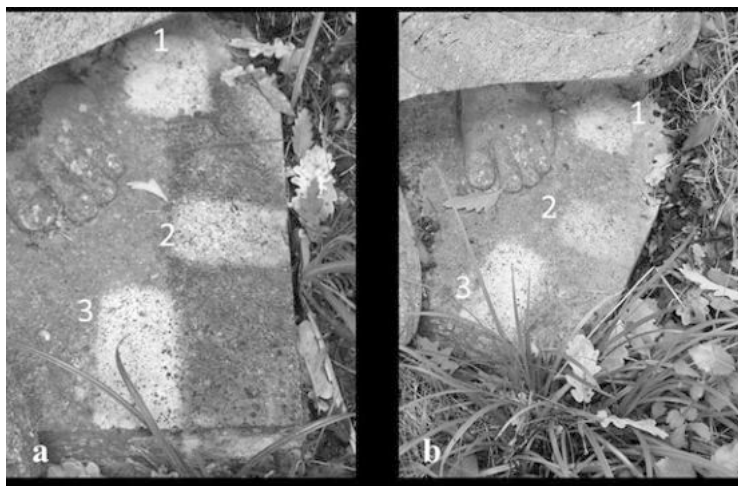
Fig. 11.4 Biofilm removal on the stone pedestal of a statue in the Vatican Gardens. The products were applied in cellulose pulp, (a) the surface after the cleaning with 1- BioZ; 2- water; 3- LIQ 3%. (b) the same surface 18 months after the treatments: the portion cleaned with water (2) shows a new biofilm growth, while the portions treated with BioZ and LIQ are still clean
